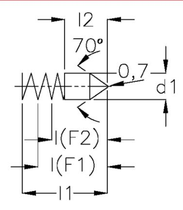
$\begin{array}{ll} d1 & = 3.0 \\ I(F1) & = 9.0 \\ I(F2) & = 6.7 \\ I1 & = 11 \\ I2 & = 5.2 \\ Spring pressure (F1) N = 1.6 \\ Spring pressure (F2) N = 3.4 \\ \end{array}$
